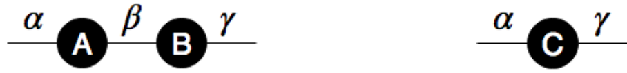
(a) Contraction of two tensors A_{\alpha,\beta} and B_{\beta,\gamma} by the index \beta . (b) Contraction result.
