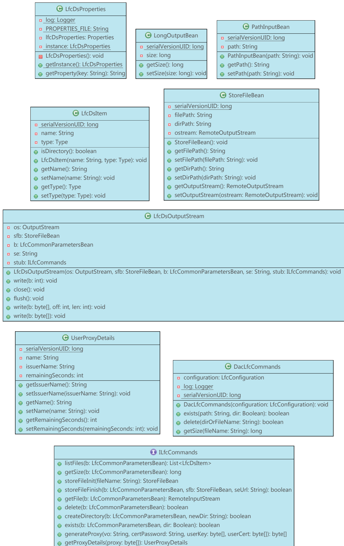
Figure 44: Class diagrams: LfcDsProperties, LongOutputBean, PathInputBean, LfcDsItem, StoreFileBean, LfcDsOutputStream, UserProxyDetails, DacLfcCommands and ILfcCommands.
