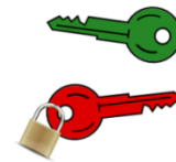
Figure 4. Public and private key. The private key should be kept secret and be only known to the owner, whereas the public key may be widely distributed.
