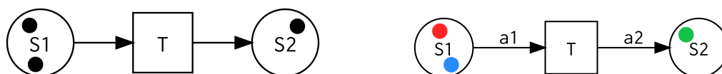
(a) Petri net. States (circle nodes) contain tokens (black dots). There is one transition \tau between states S_1 and S_2 .
