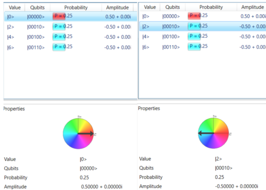
Figure 15: The state of the system exactly in the moment lineated in figure 14. QuIDE can give users information about value of the registers, states of qubits, probability and amplitude. It also displays amplitude as a vector in a complex plane. The left part of the figure shows amplitude on a complex plane of the first state (highlighted in blue) and the right part - of the second state. Directions of arrows are inverted.
