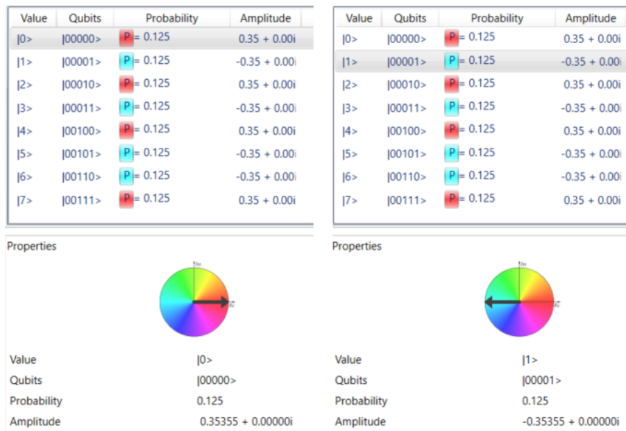
Figure 24: State of the system in the moment lineated in figure 23. QuIDE can give users information about value of the registers, states of qubits, probability and amplitude. It also displays amplitude as a vector in a complex plane. The left part of the figure shows amplitude on a complex plane of the first state (highlighted in blue) and the right part - of the second state. Directions of arrows are inverted.
